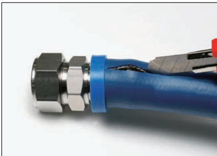
1. Slit hose lengthwise from blue finishing cap to end of barb. Do not damage barbs.
