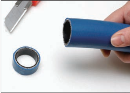
1. Cut a clean, square edge on end of hose
