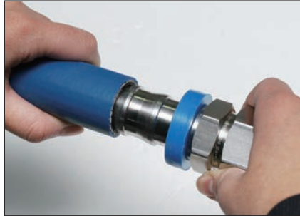
2. Cover first barb of end connection with hose. (Lubrication fitting stem with light oil may ease assembly)
