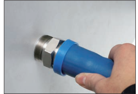
3. Hold end connection against flat surface, Grip hose and push with a steady force until hose seats into blue finishing.
